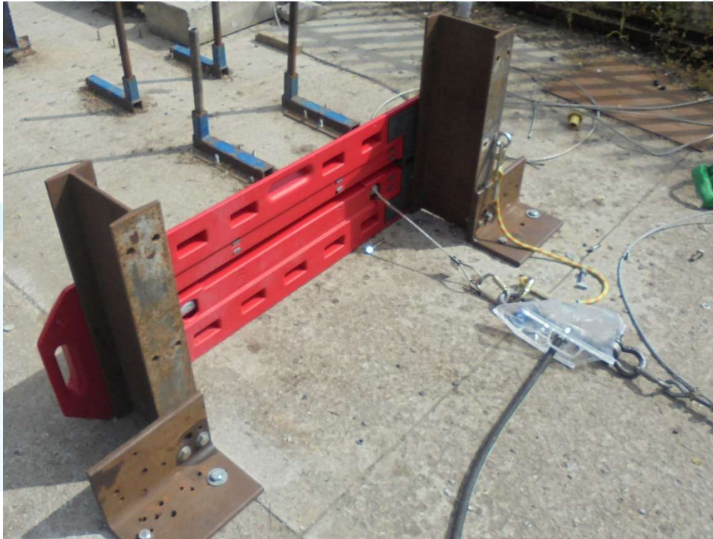
Figure 2 – Anchor device described as “Gridmesh” in test setup
